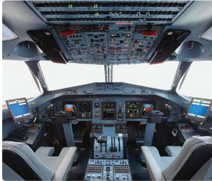
A new glass cockpit comes with a completely new avionics suite.
